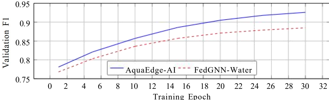
Figure 2: Validation performance curves. AquaEdge-AI converges faster and reaches a higher plateau, suggesting improved optimization stability under noisy telemetry.
